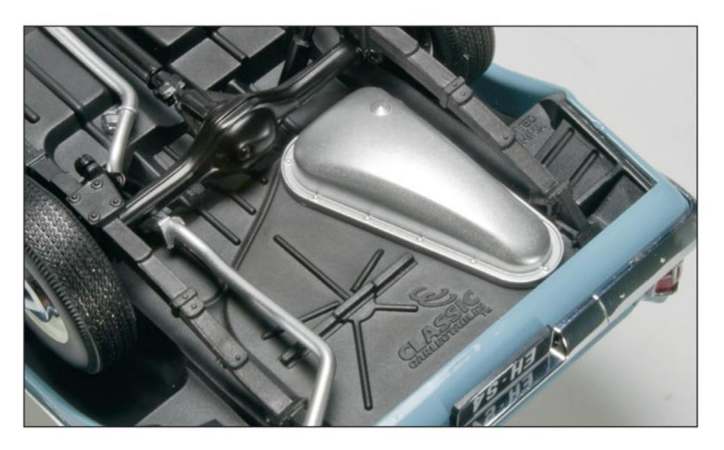
Part of the S4 option package was a larger 12 gallon fuel tank that was a straight swap with the original factory tank.
